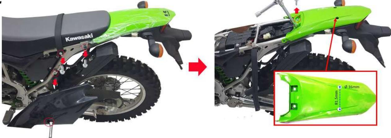
Open the seat , remove the original bolt then cut out the pattern include in the 2nd page user guide . Place in to rear fender and make 4 Ø 16mm holes in the marks
