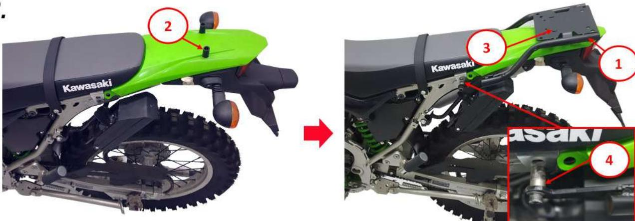
Install part no.2 in to rear fender holes, then install fitting kits no.1 in to motorbike using part no.3 and no.4
